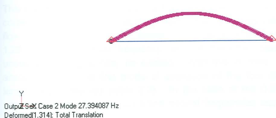
Figure 2.9: Mode shape of tube with length 1.2675 m with pinned supports
