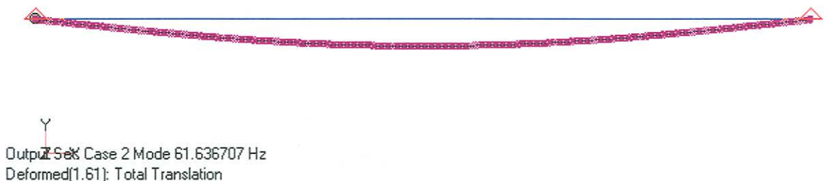
Figure 2.7: Mode shape of tube with length 0.845 m
