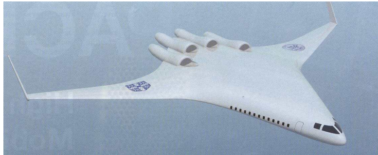
Figure 2.12: The Blended Wing Body Concept from Cambridge University (Anonymous, 2005:12).
