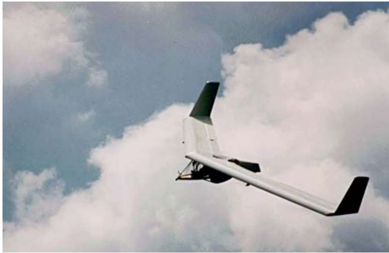
Figure 2.11: The SWIFT foot launched glider. (Kroo et al., 1991)
