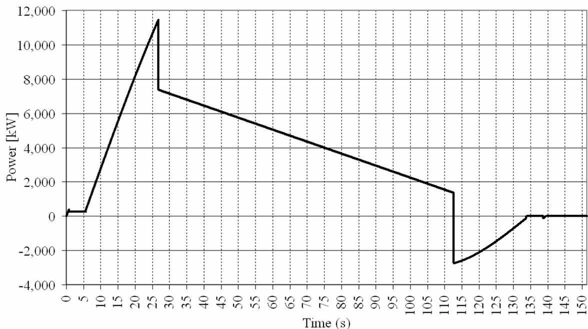
**Figure 2.2: Modelled active load profile for a single hoist cycle of rock winder.**
