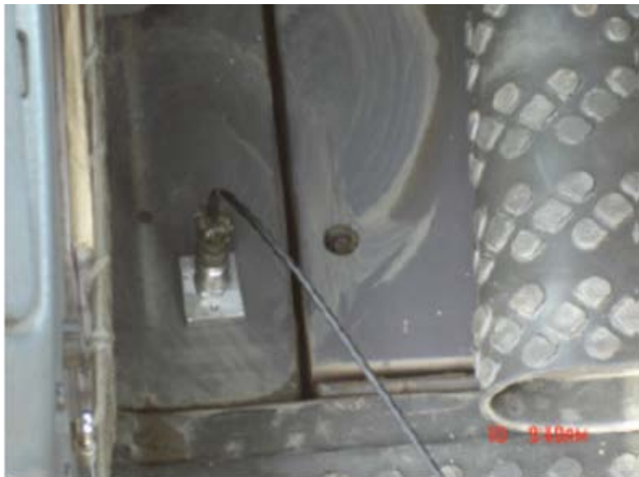
Figure 2.4: Floor ICP industrial accelerometer
