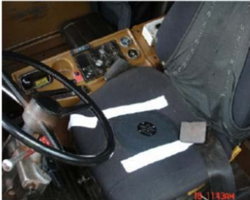
Figure 2.3: Dytran tri-axial seat accelerometer
