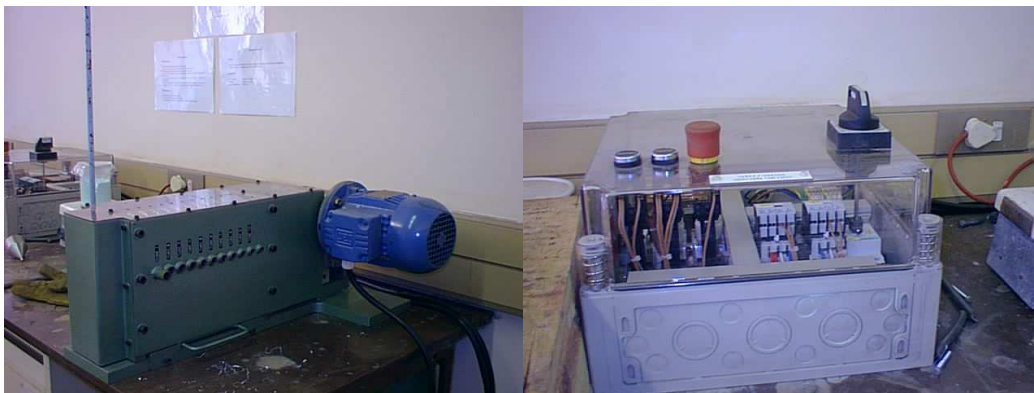
Figure 6-2: Tube Roller and Motor Control Box
