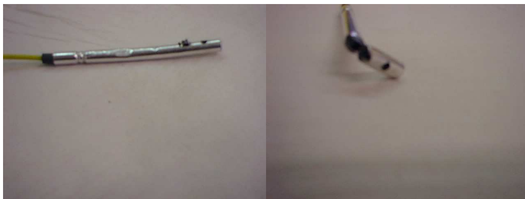
Figure 6-14: Examples of Detonator Assemblies that Ignited and Burned
