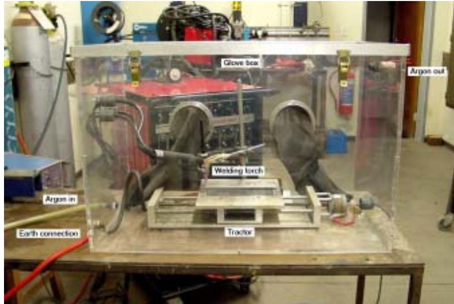
Figure 3.1 Experimental arrangement for autogenous welding.
