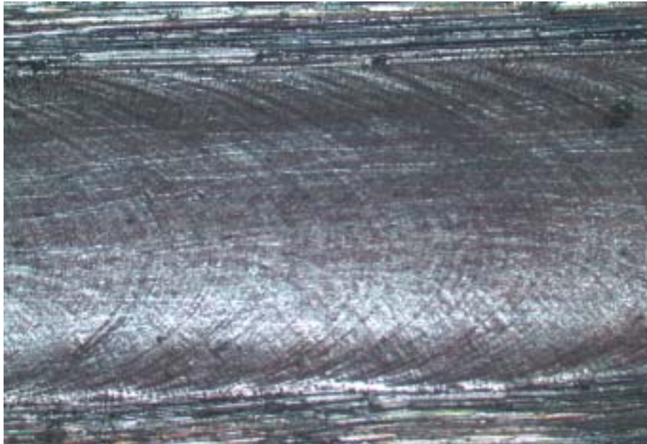
Figure 4.2 Surface appearance of VFA 752 (low N, high S) welded in pure argon. Magnification: 8x.
