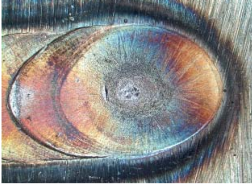
Figure 5.2 The end crater of a weld bead. Magnification: 10x.
