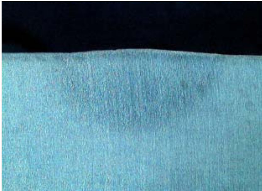
Figure 5.3 A cross section of a weld bead. Magnification: 10x.
