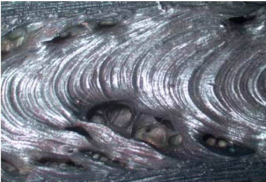
Figure 4.4 Surface appearance of VFA 752 (low N, high S) welded in an Ar-24,5%N 2 shielding gas atmosphere. Magnification: 8x.
