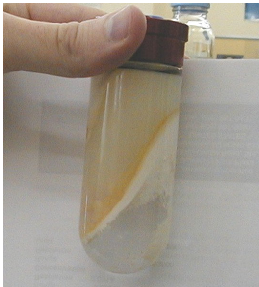
Figure 3-26. Photograph of centrifuge tube containing separated PFOB, after 96 hours of centrifugation at 60 000 g's. A layer of sediment has formed at the water-PFOB interface during centrifugation, consisting of emulsion (bottom) and lecithin (top).
