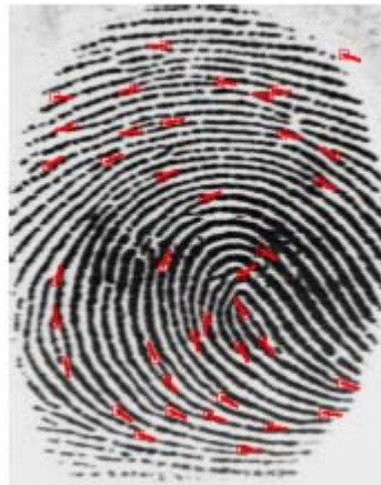
Figure 3-2 A fingerprint gathered using a solid-state sensor with the minutiae marked in red [13]. Reprinted under permission [13].
