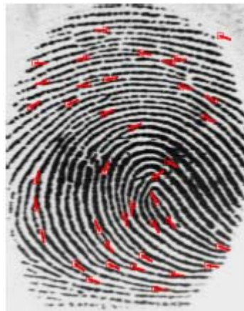
Figure 3-2 A fingerprint gathered using a solid-state sensor with the minutiae marked in red [13]. Reprinted under permission [13]. (Refer to the Appendix 1 for a colour version of the figure)
