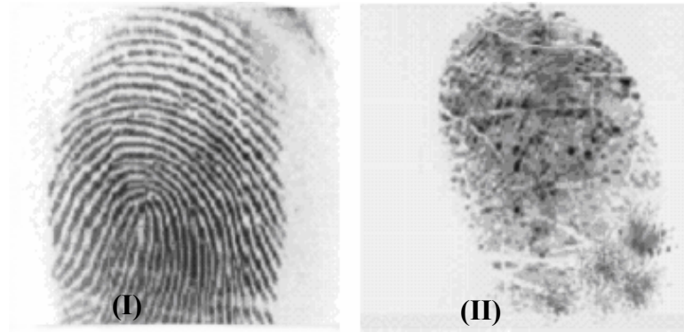
Figure 2-1 An example of (I) a normal fingerprint will be ideal for use in fingerprint recognition, and (II) a damage fingerprint as one can see most of the grooves are missing and you do not really get any pattern except for the scar lines.
