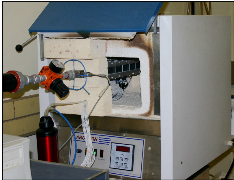
FIGURE 3.4: Furnace used to control the experimental channel wall temperature
