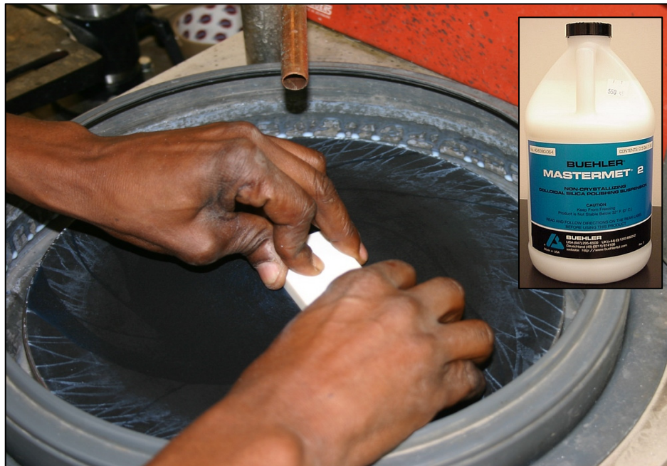
FIGURE 3.6: Final polishing stage of the substrate surface (Insert: Silica suspension)
