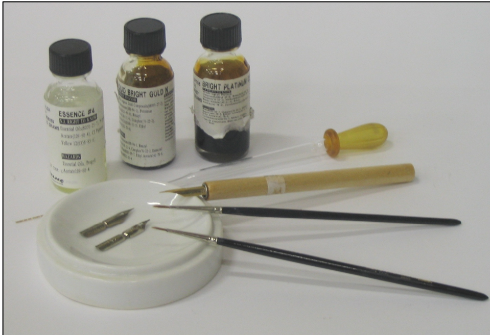
FIGURE 3.7: Platinum, gold and thinning essence solutions along with stylus, brushes and other utensils used during gauge application
