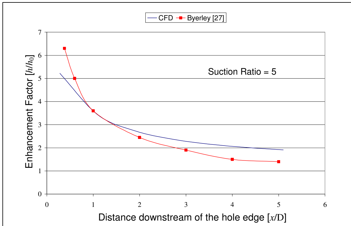
FIGURE 5.14: Centre-line heat transfer enhancement factors downstream of the 90^\circ extraction hole
