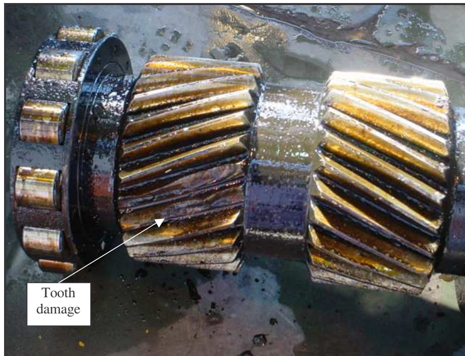
Figure 4.10: Tooth damage on the left gear set of the monitored pinion.
