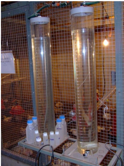
Figure 2.1 Calibrated 15 L Perspex cylinder
