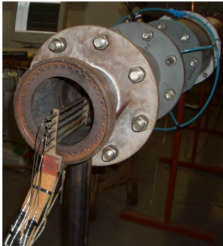
Figure 70: The five K-type thermocouples in a rake at the combustor outlet
