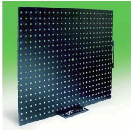
Figure 53: A black and white calibration target [21]
