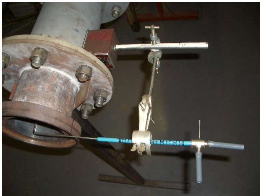
Figure 72: A magnetic clamp holds the Pitot tube onto the test rig in the correct position
