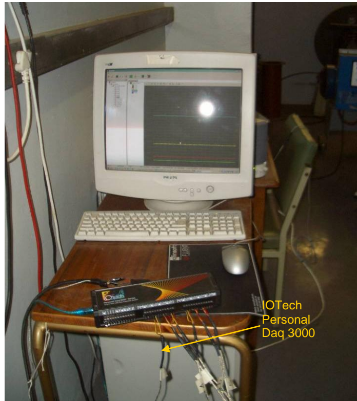
Figure 71: The data acquisition system and computer used for thermocouple measurements
