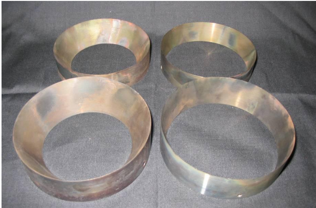
Figure 76: The 30% (left) and 10% (right) primary and secondary zone wedge rings
