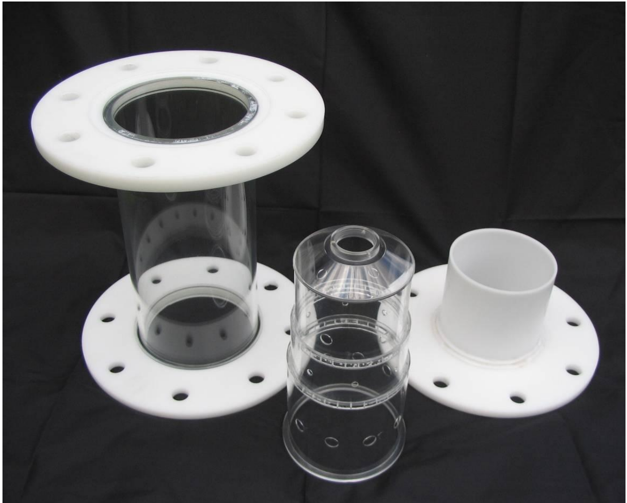
Figure 73: The transparent combustor parts - casing, liner and outlet pipe
