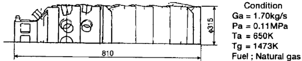
Figure 30: Mandai and Nishida's combustor configuration and conditions for the diffusion flame combustor [7]
