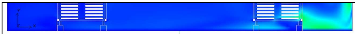
Figure 6-9 Detail view of the speed contour in the YX-plane at the centre of the inlet vent
