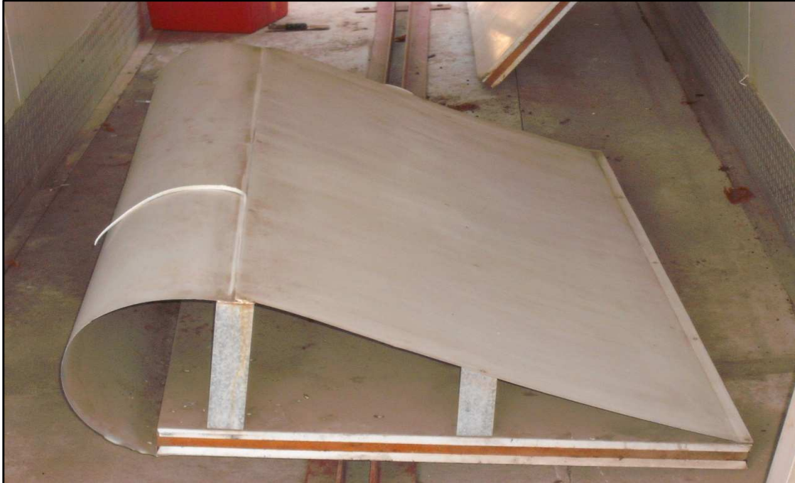
Figure 4-25 Side view of flow diverter showing supporting struts
