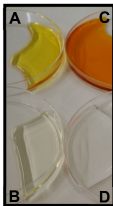
Figure 2.4. Illustration of the catalytic activity of peroxidases to oxidize the substrate, o -phenylenediamine dihydrochloride (colourless solution) to 2,3-diaminophenazine (orange solution) in sodium citrate buffer with H 2 O 2 . A: Extracted soluble protein fraction, B: Extracted bound protein fraction, C: Positive control and D: Negative control.
