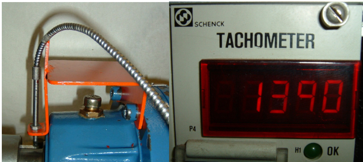
Figure 3.4 - One pulse per revolution speed display system
