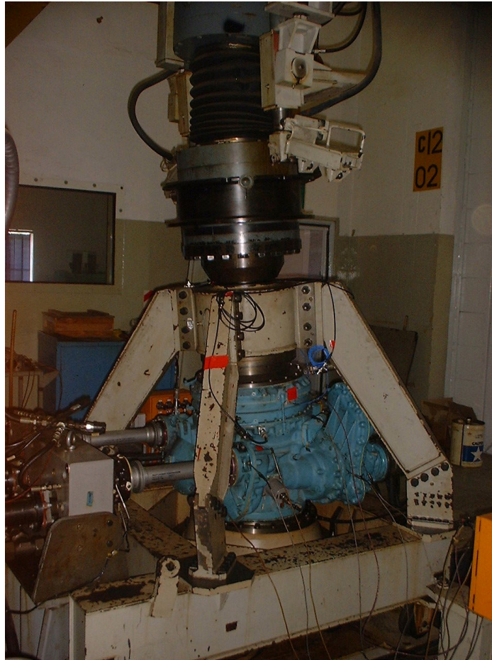
Figure 2.1 - Oryx gearbox during testing on test bench
