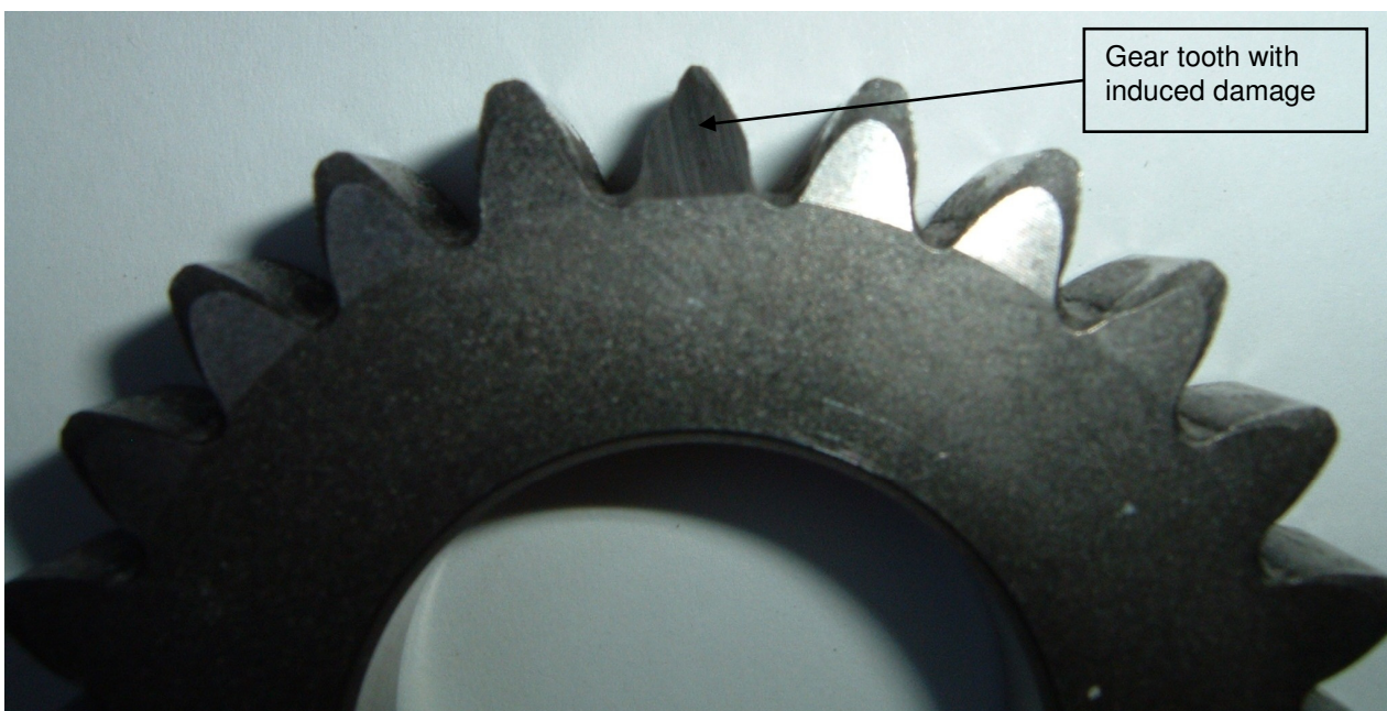
Figure 3.6 - Induced damage on a planet gear tooth
