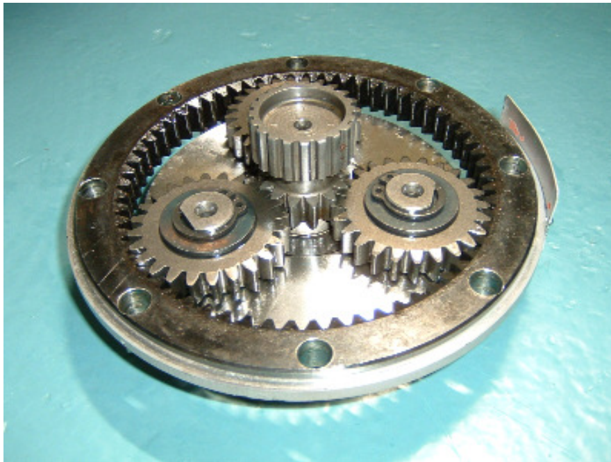
Figure 2.3 - Gears of the gearbox
