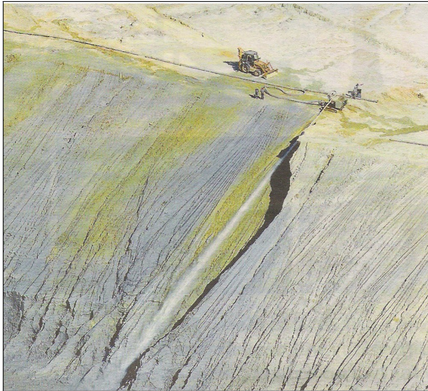
Figure 41: A gold dump being recycled by DRDGold, West Rand, 2012. ( The Citizen CitiBusiness 2012:18).
