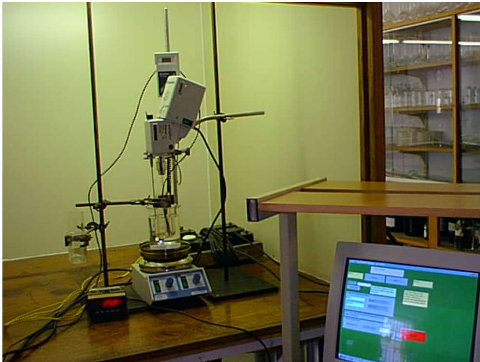
Figure 3.1 Schematic Of Cooling Curve Measurement Setup.
