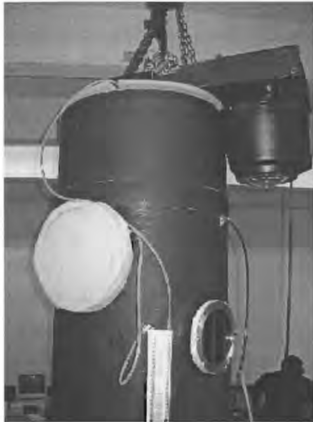
Fig 5.6 Upper part of the vacuum vessel with the motor for the compressor. The inverted orientation of the motor is to get the correct sense of rotation of the impeller.
