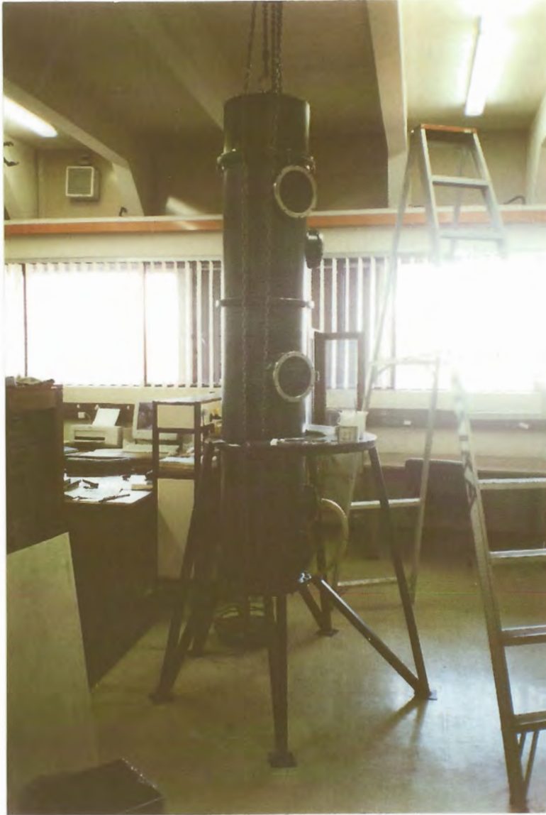
Fig 5.4 The uninsulated 2.35m tall vacuum vessel showing 200mm windows, stand and scaffolding. The pulley block is used to raise and lower the small top compartment (housing the turbo centrifugal compressor, and at a pressure p + \Delta p above that of the main compartment).
