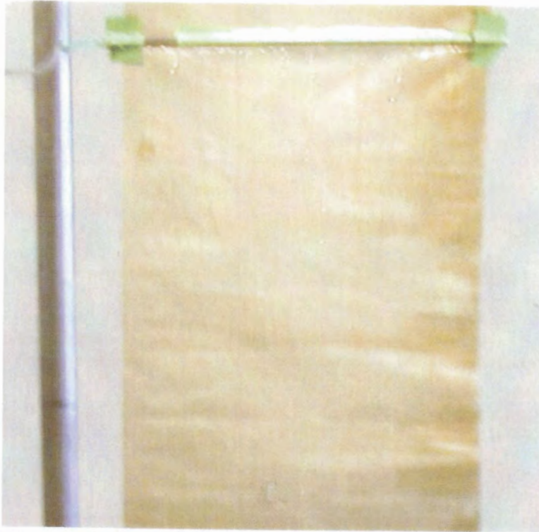
Fig. 6.10 Sulfonated film with water flowing on its surface.
