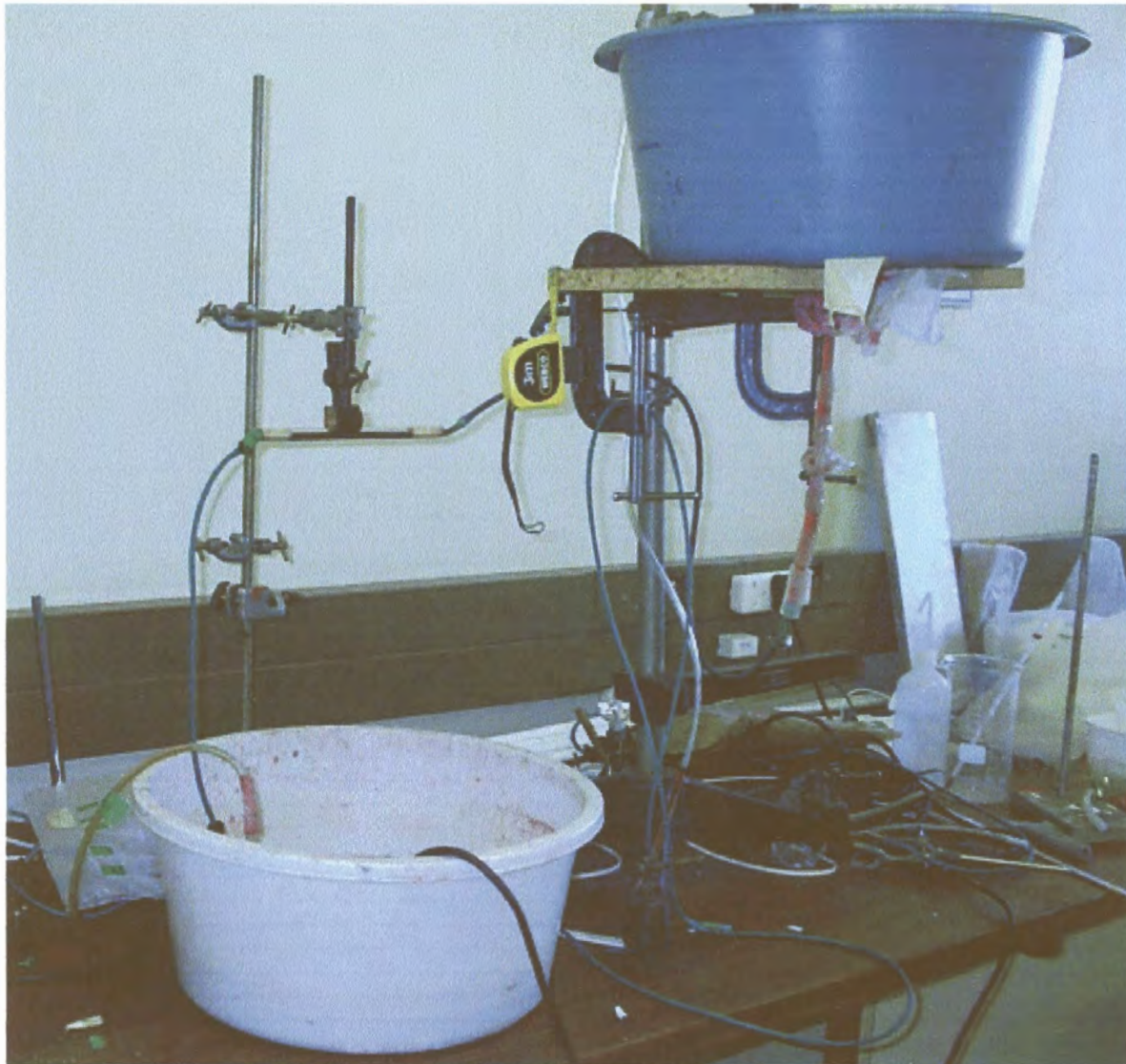
Fig. 6.17 Setup for liquid distributor testing.
