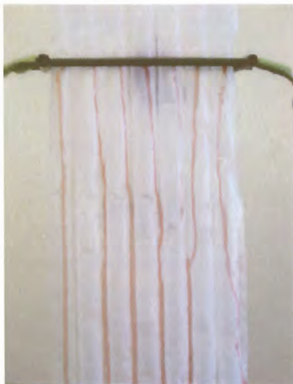
Fig. 6.9 Flow dripping through the weld lines of an oxyfluorinated film.
