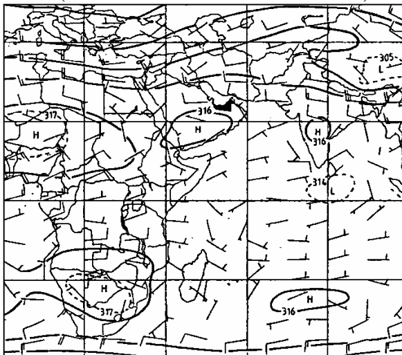
Figure 3.9. April mean 700 hPa circulation. Mean wind velocity in knots (each full barb = ten knots = 5\text{ms}^{-1} ).
