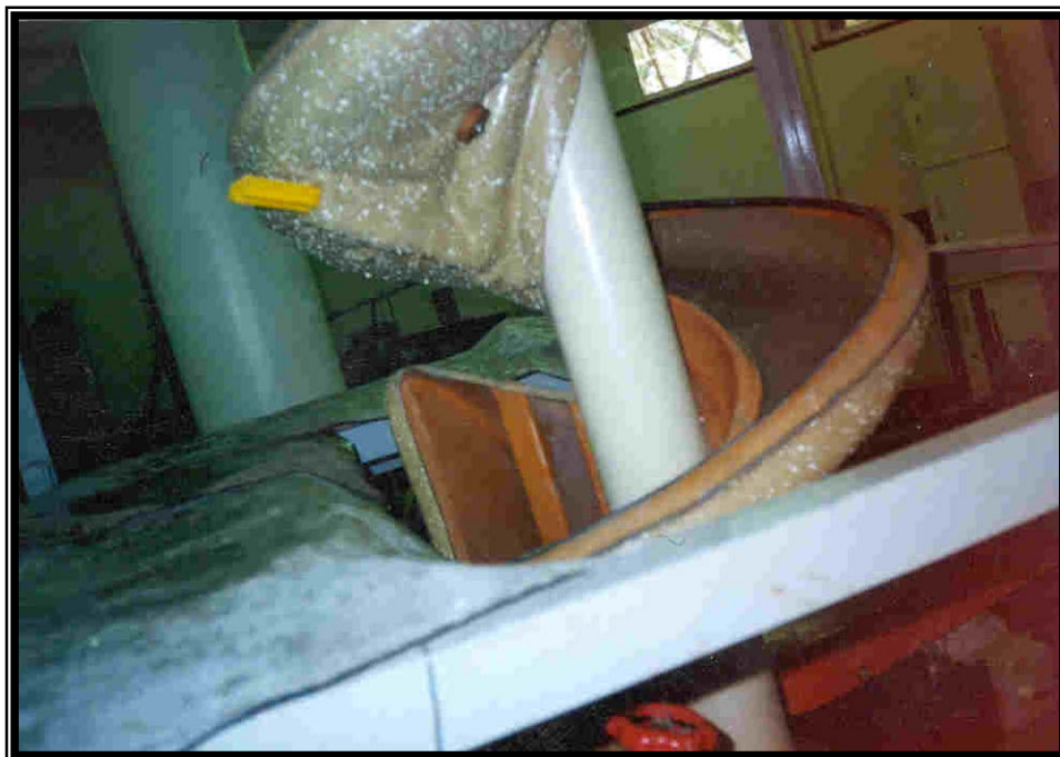
Figure 16. A photo of the spiral used for gravity separation.
