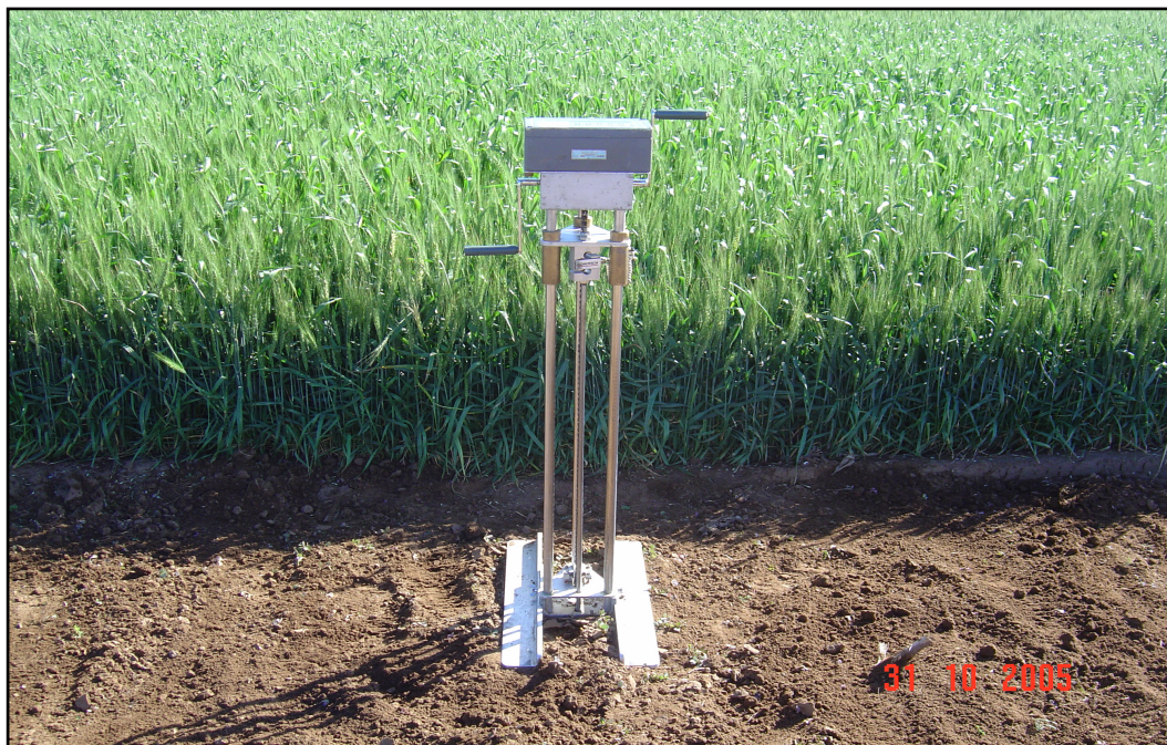
Figure 3.5: Penetrometer used for measuring the degree of soil compaction on a farm
