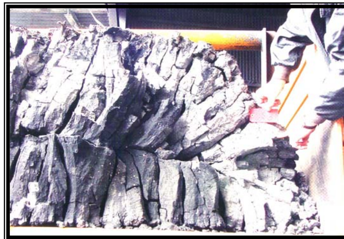
Figure 8: Close up of coke piece B from the bottom of the coke bed.
