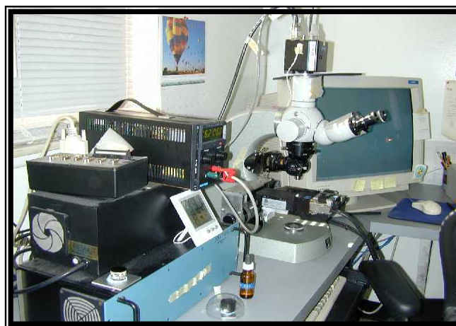
Figure 13: Microscope and computer set up with automatic stage and stepper motors for scanning the coke.
