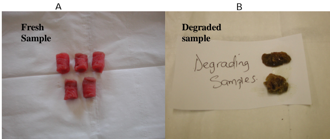
Figure 4.1.1. Fresh samples of 2.0g on day 0, before exposure to the environment and degraded samples in day 15.
