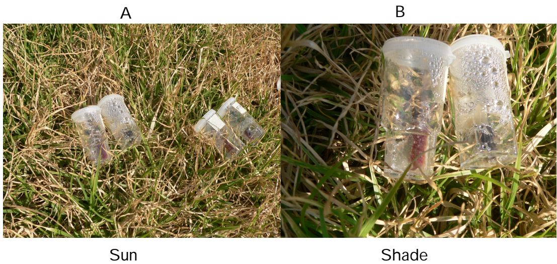
Figure 4.1.2. The degradation of samples during winter from the shade and the sun on day 15 as compared to the fresh samples (Figure 4.1.1).
