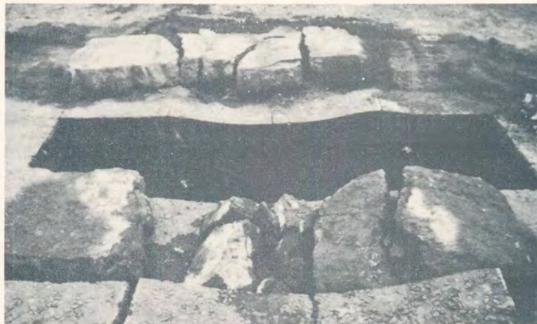
(b) Note the relatively smaller blocks of recovered upper stabilized subbase material, due to fatigue cracking and fracturing. The lower stabilized subbase experienced only fatigue cracking, hence the bigger blocks of material.
