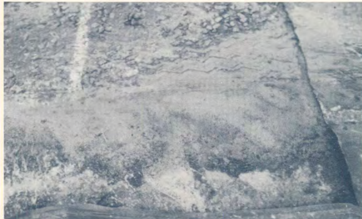
(c) Fines on the side of the test section after the "saturated" test.
