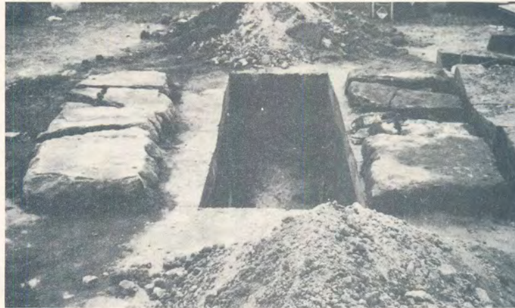
(a) General view of the recovered blocks of subbase material. Upper subbase on the right, lower subbase on the left.
