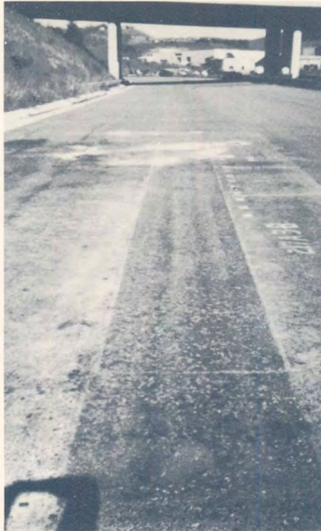
(a) General view of the surface of Section 2 (217A3) after 32 \times 10^6 E80s in the dry state.
