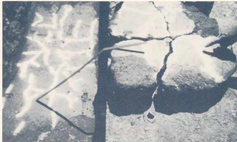
(b) Printed crack pattern of the bottom of the lower stabilized subbase on the top of the unexcavated selected subgrade layer.
