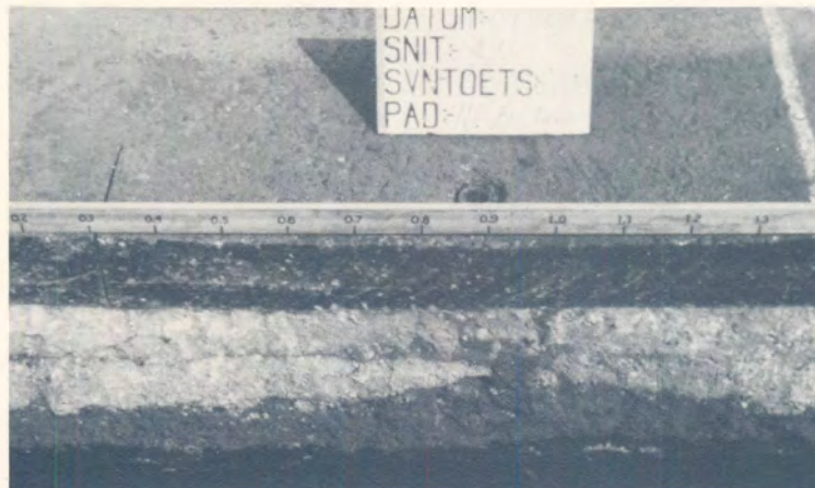
(a) Face of the test pit, indicating the moisture regime at the position of the crack (point 1,0 on straight-edge). The light brown colour is the well-stabilized weathered Granite subbase layers.
