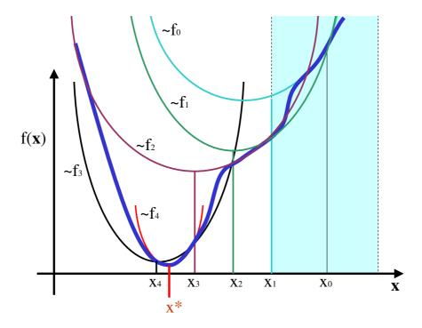
Figure 2.1: Simplified illustration Dynamic-Q progresses on how optimisation iterations
