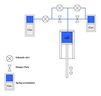
Figure 1.1:  $4S_4$  Suspension Unit
