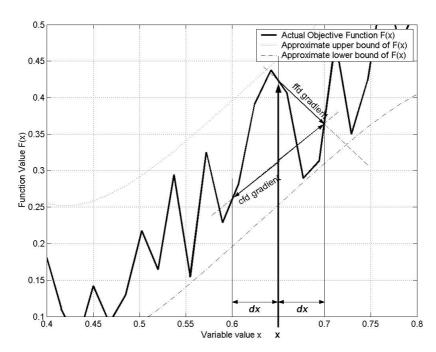
Figure 2.2: Finite difference gradient approximation methods
