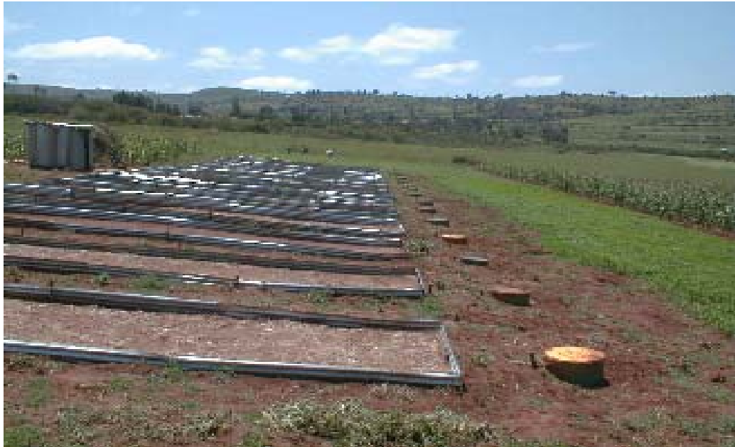
A. Experimental setup of the runoff plots
