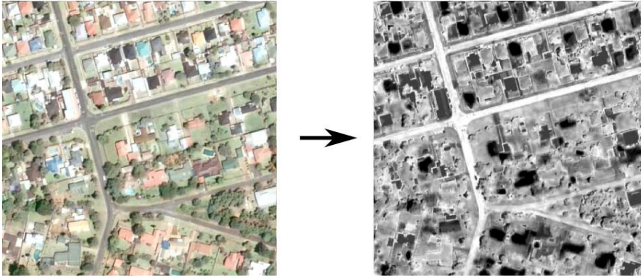
Figure 2.2: An example of spectral classification through classical statistics
