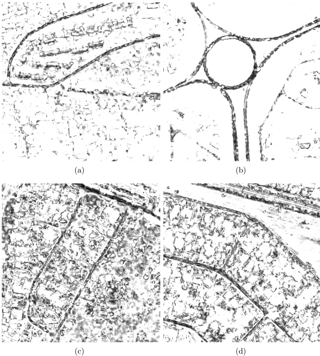
Figure A.12: Fully automated spectral classification (excluding the k-means filter)
