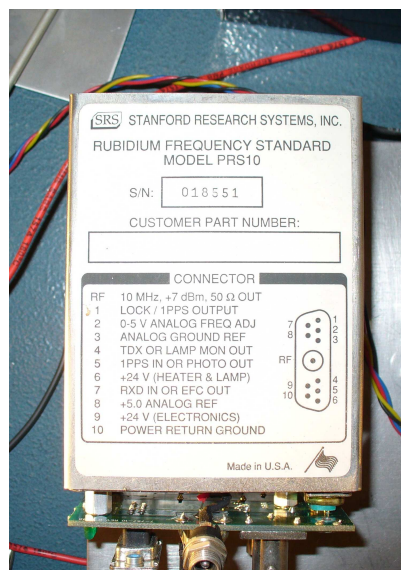
FIGURE 4.10: Rubidium frequency standard
