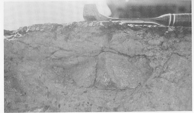
(a) Final crushed state (compression failure) in the top 50 mm to 75 mm of the cemented base layer, after testing in relatively dry conditions.
