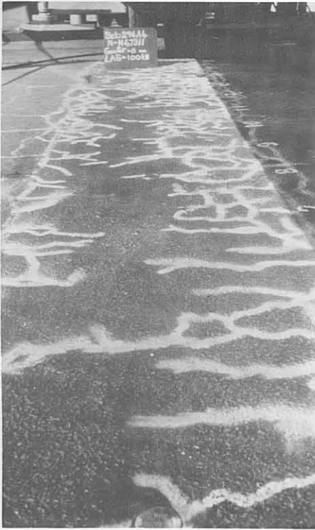
(a) Relatively fine cracking after 1,44 \times 10^6 100 kN repetitions.
