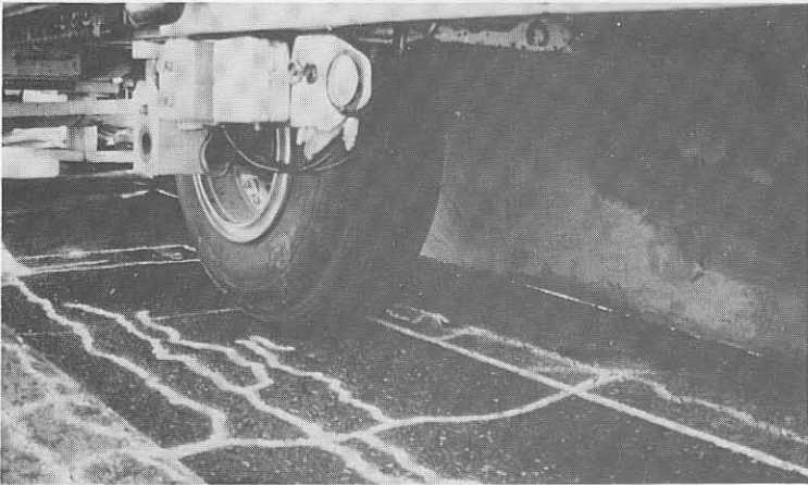
(b) Fatigue cracking and deformation (approximately 40 mm) after 11 331 repetitions of a 150 kN, 1445 kPa single aircraft wheel load.
