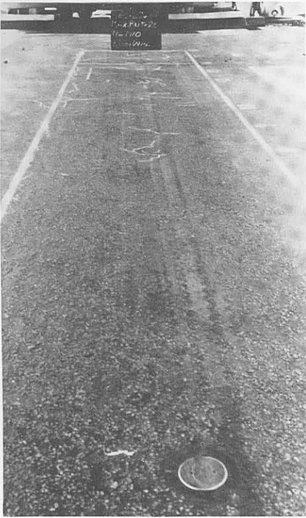
(a) Condition before testing; some fine cracking evident from measuring points 9 to 15 at the start of the test.
