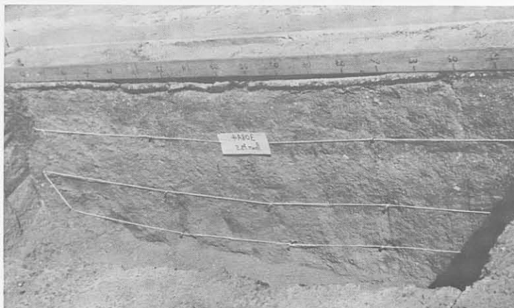
(c) Final deformation (approximately 24 mm) at measuring point 13,5 after approximately 2,64 \times 10^6 100 kN repetitions.
