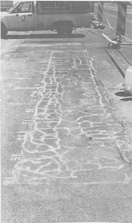
(b) Final fatigue cracking and crushing after approximately 2,64 \times 10^6 100 kN repetitions.
