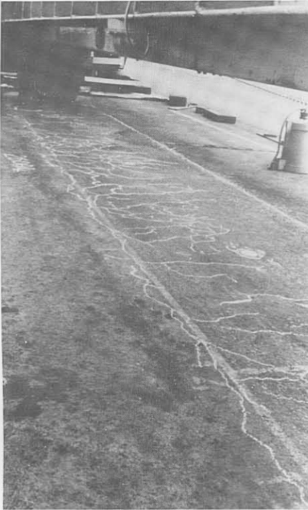
(a) Relatively fine crack pattern after 1,95 \times 10^6 repetitions (E80s). Note the waterbottels for introduction of depth water (20 mm to 450 mm) on the side of the section at measuring positions 9 to 15.
