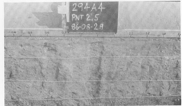
(c) Relatively low deformation (approximately 10 mm) after testing in the relatively dry conditions on Section 294A4.
