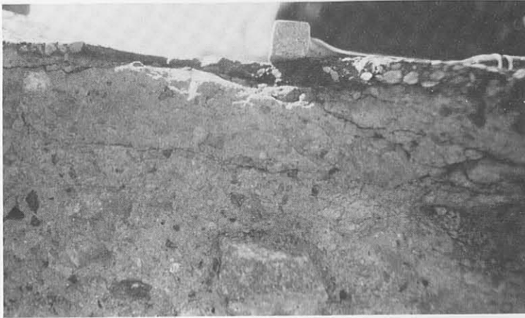
(a) Final crushed state (compression failure) in the top 50 mm to 75 mm of the cemented base layer, after testing in relatively dry conditions.
