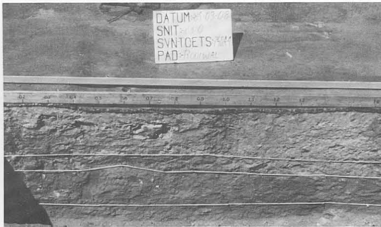
(b) Approximately 20 mm deformation after 2,4 \times 10^6 repetitions (E80s).
