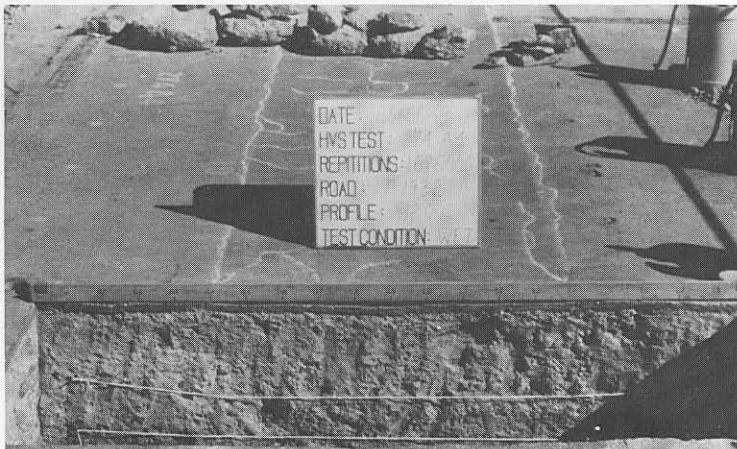
(b) Deformation less than 8 mm at end of test.
