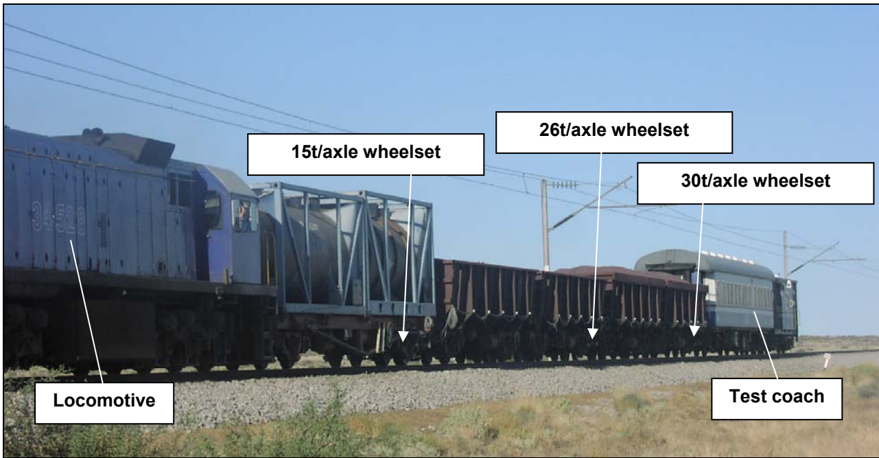
Figure 4-35: Test train setup with three instrumented wheelsets at Iron Ore Export line tests
