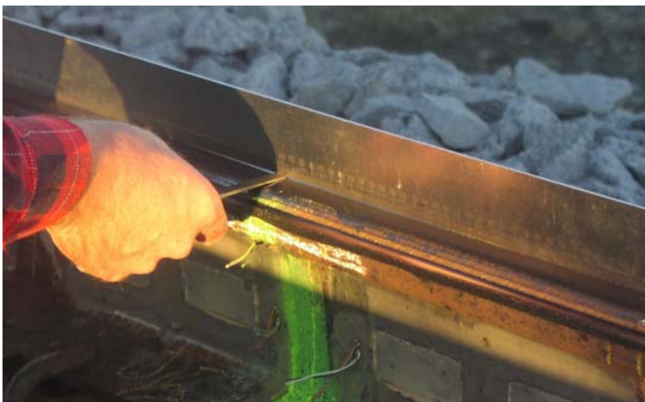
Figure 4-4: Measuring the depth of a dip joint (soft flash butt weld)
