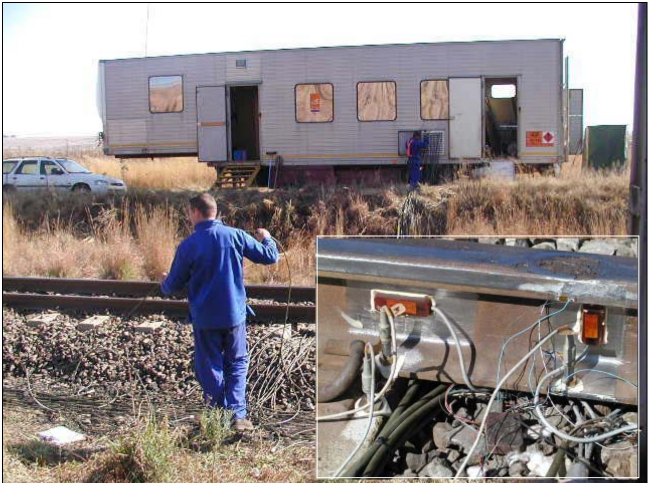
Figure 4-16: Spoornet mobile laboratory for measuring strains, deflections and accelerations.
