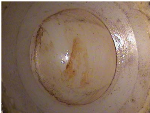
Figure 6.32 – No deposit was present on the balls retrieved from the stations using the synthetic lubricant as test medium.
