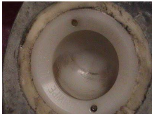
Figure 6.35 – The retrieved cup from the second station using the synthetic lubricant clearly shows the wear pattern.
