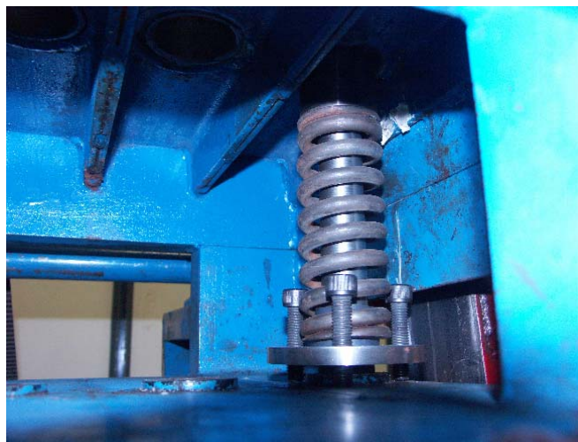
Figure 6.6 – Every station was mounted on a spring configuration to supply the required load profile.
