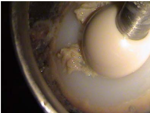
Figure 6.22 – The “seal” in station 4 after 4 000 000 cycles.
