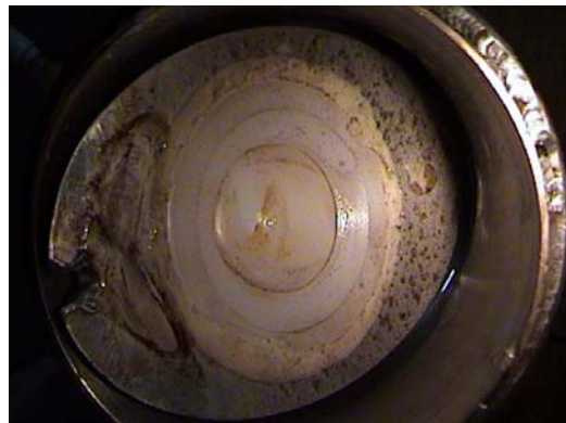
Figure 6.33 – No deposit was found in either of the two stations using the synthetic lubricant.
