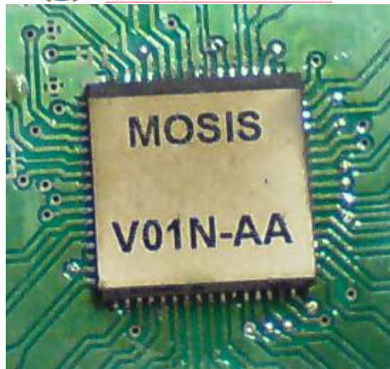
Figure 6.11. Photo of the 64 pin QFN packaged IC mounted on the test PCB.
