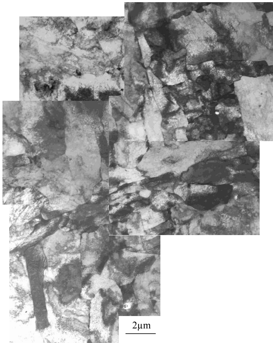
Figure 8.16 Acicular ferrite morphology in alloy #5 after fast cooling of 47^{\circ}\text{C s}^{-1} after the hot rolling process.
