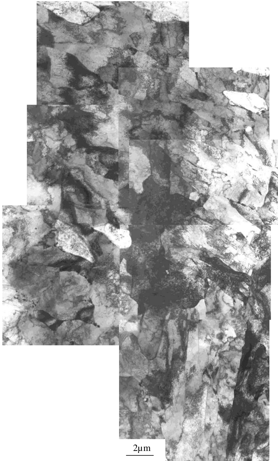
Figure 8.11 Thin foil TEM composite micrographs of the acicular ferrite in alloy #4 after a rapid cooling rate of 47\text{ }^{\circ}\text{C}\text{s}^{-1} after the hot rolling process.
