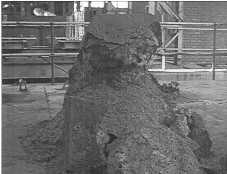
Figure 64: Front view of a slag block (tap 68) that had decrepitated
