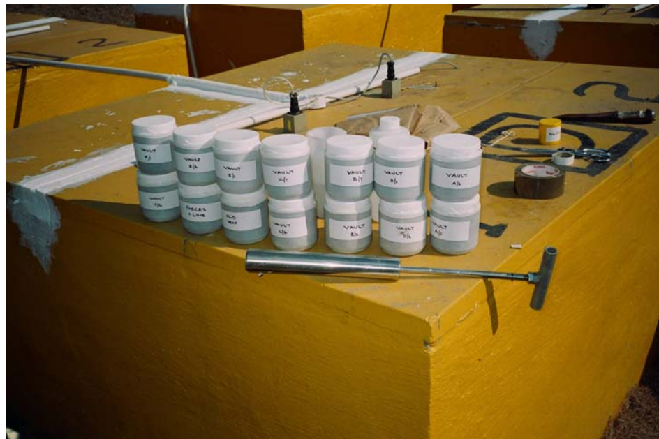
Figure 5.10: Coring device and sample bottles
