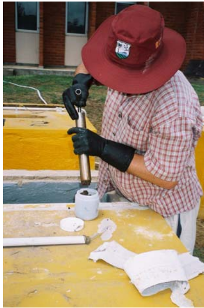
Figure 5.11: Expressing the cored material into the sample bottle
