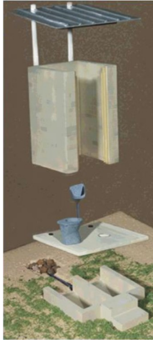
Figure 5.3: Exploded view of the eThekwini urine-diversion toilet (Photograph: eThekwini Water Services)
