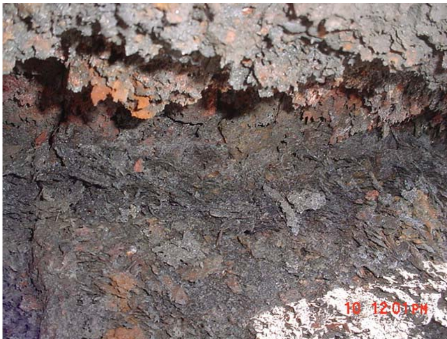
Figure 9 Example of decrepitated material showing the flake-like structure which captures air to form an isolating layer round the block when left to accumulate.
