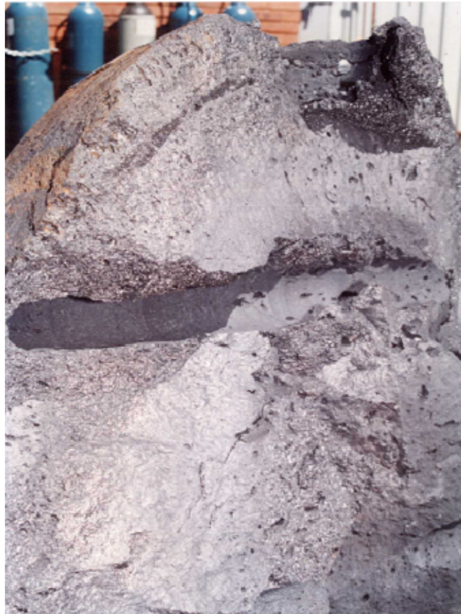
Figure 46 Cross section of block 60 showing the horizontal groove where the drill core was removed. The block surface is apparent from the rusty coloured area in the upper left hand corner of the photo.
