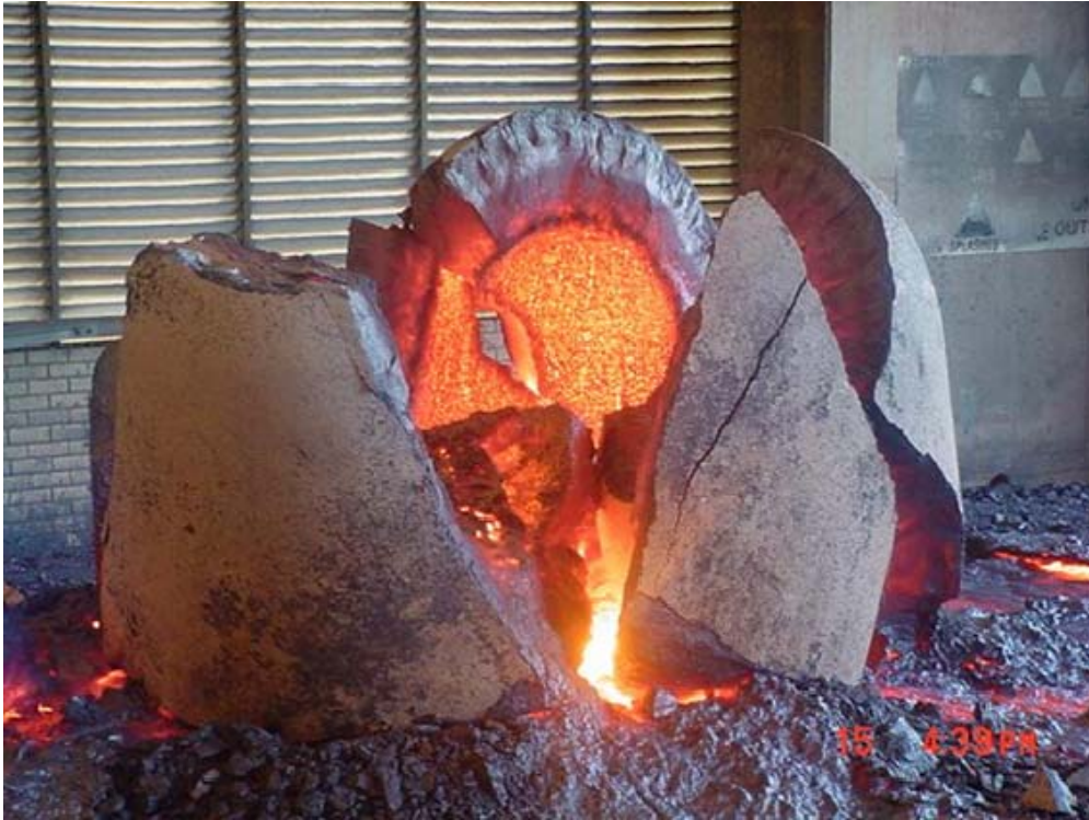
Figure 92 Internal structure of a partially solidified block, as revealed by failure during tipping after primary cooling in the pot.
