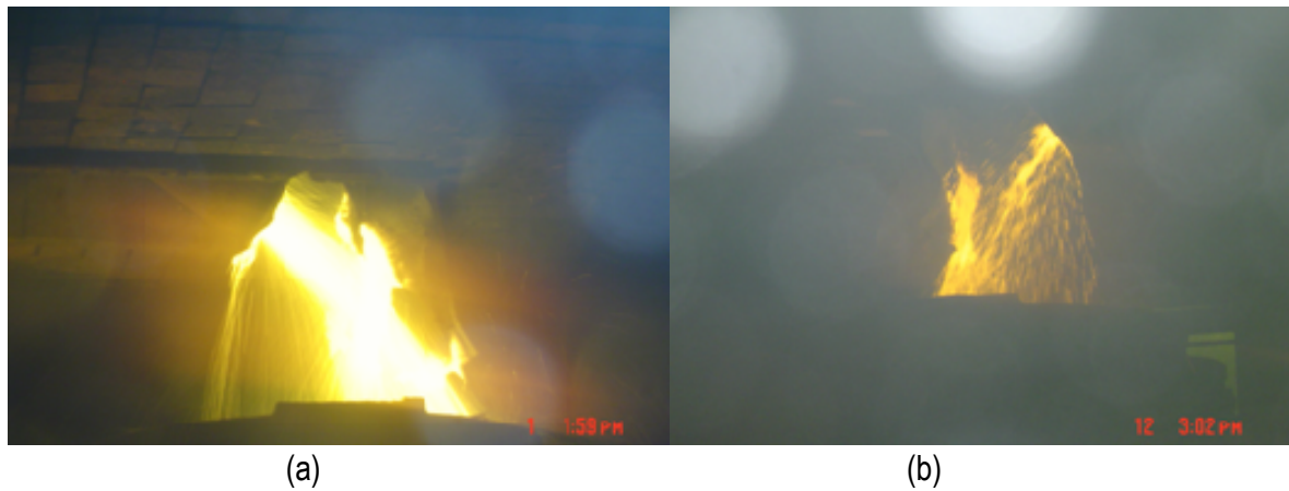
Figure 55 Photographs of the tapping stream of (a) a fast and (b) a slow tap.
