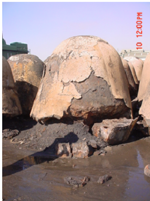
Figure 102 Photograph of a 17-18 ton slag block showing typical breaking off of the corner between the horizontal and inclined surfaces. To the left of the broken-off corner decrepitated material has formed.
