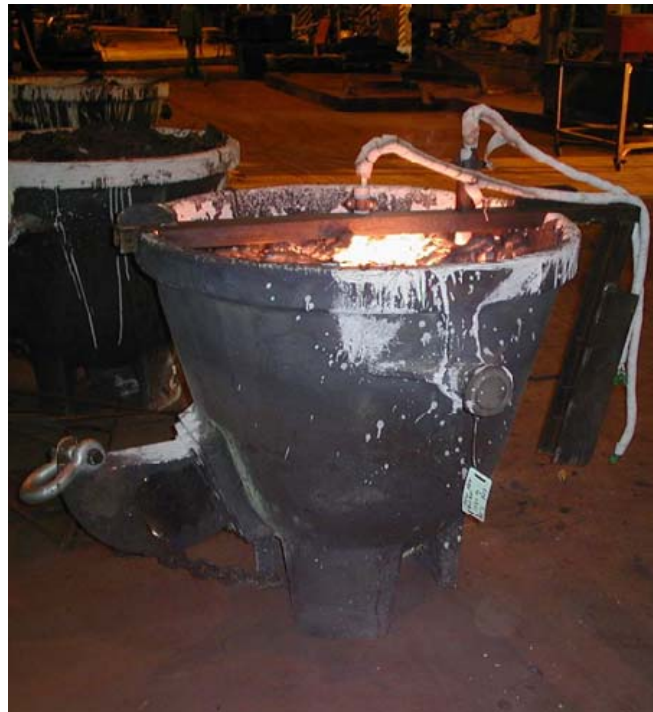
Figure 83 Photograph of a slag block and pot directly after thermocouples were inserted into the block. For support the refractory tubes were inserted into the slag through slots in a steel channel which was placed horizontally over the pot edge.
