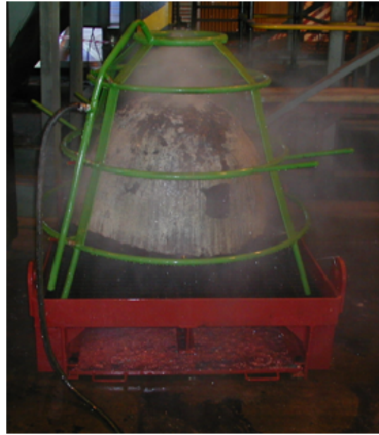
Figure 6 Slag block under water cooling during Campaign 9
