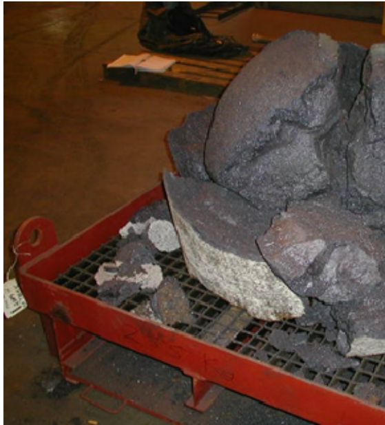
Figure 5 Grid and tray stand on which slag blocks were placed to cool
