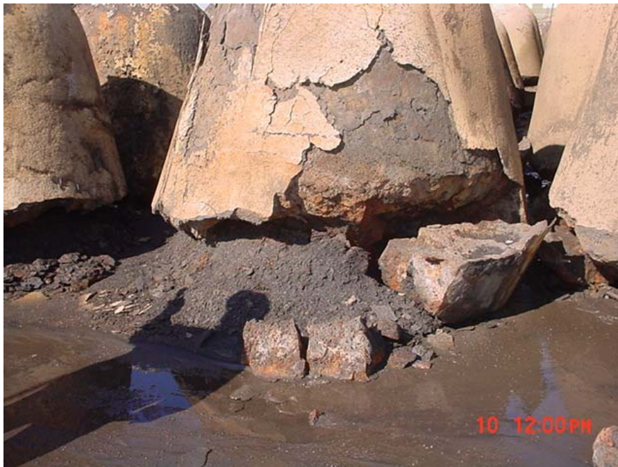
Figure 28 Photograph of an industrial-size block showing fine decrepitated material and large chunks breaking off from the block corners. As an indication of scale, the bottom diameter of the block is approximately 1.8 to 2 m.
