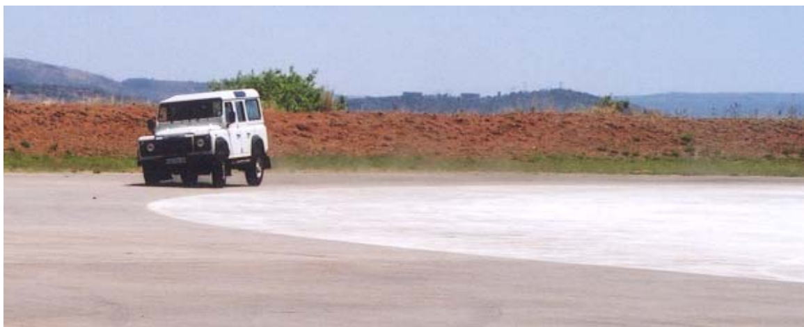
Figure 2.23 - Constant radius test
