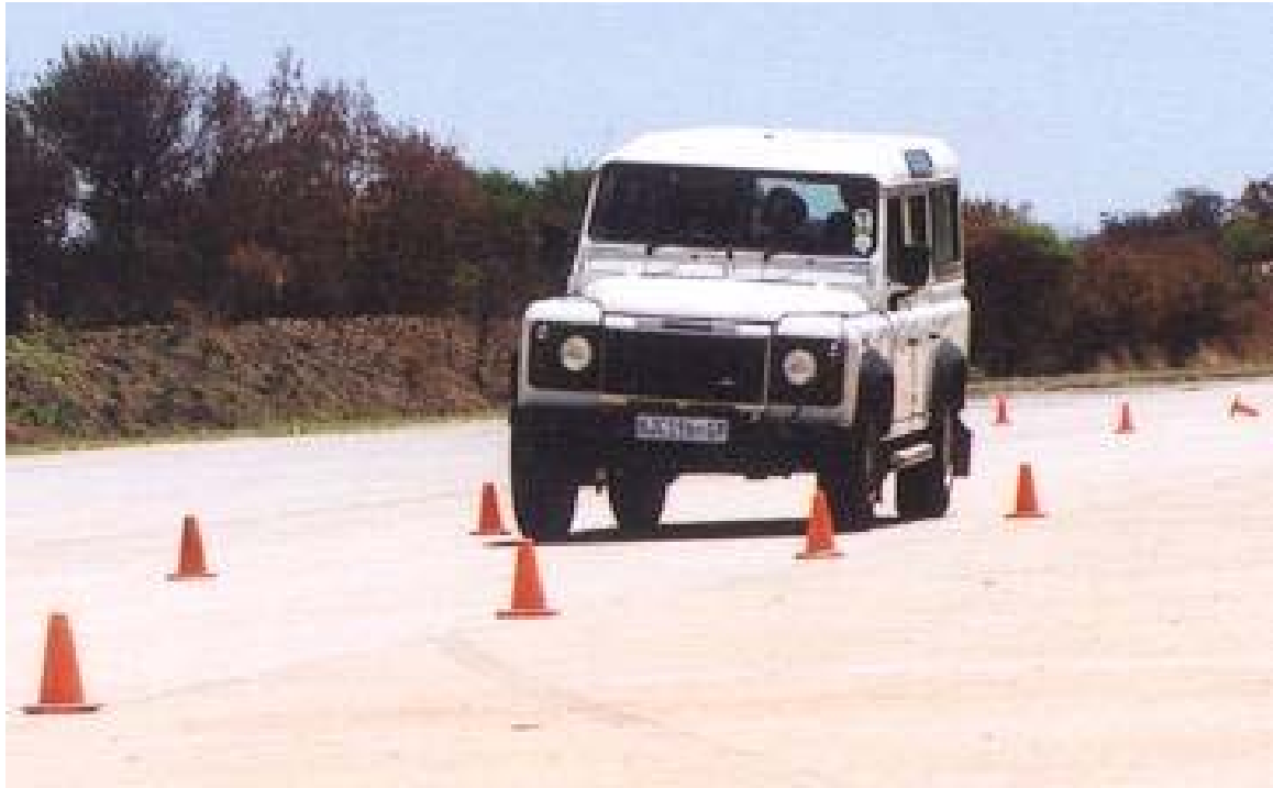
Figure 2.24 - Severe double lane change manoeuvre
