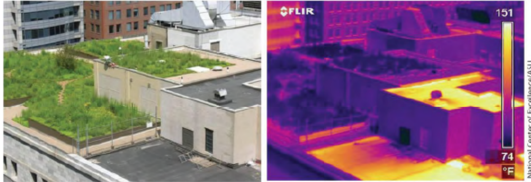
Figure 2.2. Comparative Infrared photos of an asphalt roof and a green roof “On a typical day, the Chicago City Hall green roof measures almost 40C cooler than the neighbouring roof to the right”(UHI: 2009, 22). Source: http://scpgreenbuild.files.wordpress.com/2010/10/sadhujohnston.pdf
