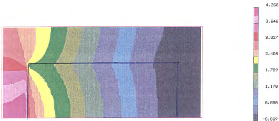
Figure 3.11 Pressure contour plot on the centre of interfin region - U_o = 1 \text{ m/s} - Laminar flow.
