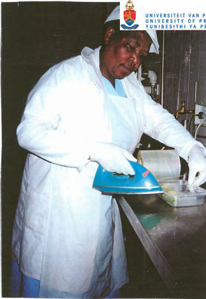
Fig. 15: Sealing of the packaging tub with a layer of polypropylene
