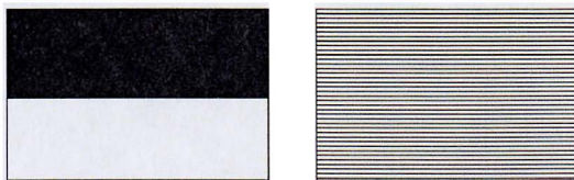
Figure 5.12: The video server can be configured to grab the even fields of the right and the odd fields of the left camera. Then both fields are assembled together in one image which will again be encoded and sent to the client. With this trick it is possible to keep a high frame rate even sending stereo images over the network.
