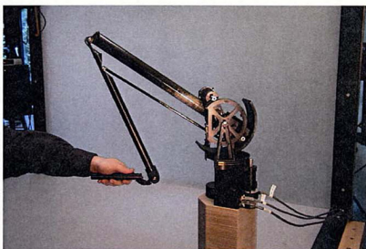
Figure 1.8: The Phantom Force Feedback Device integrated into the Responsive Workbench's interaction space. [Sensable Inc.,2001]
