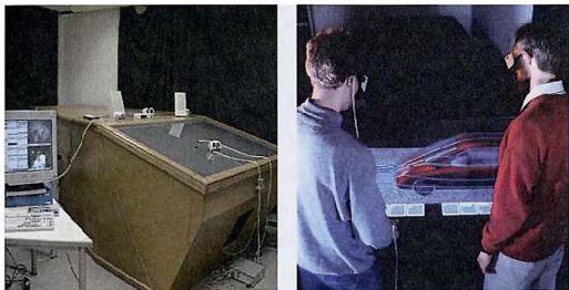
Figure 1.2: The Responsive Workbench provides a natural metaphor for visualizing and interacting with three-dimensional computer-generated scenes. On the right hand side two engineers are working collaboratively in front of the same display.
