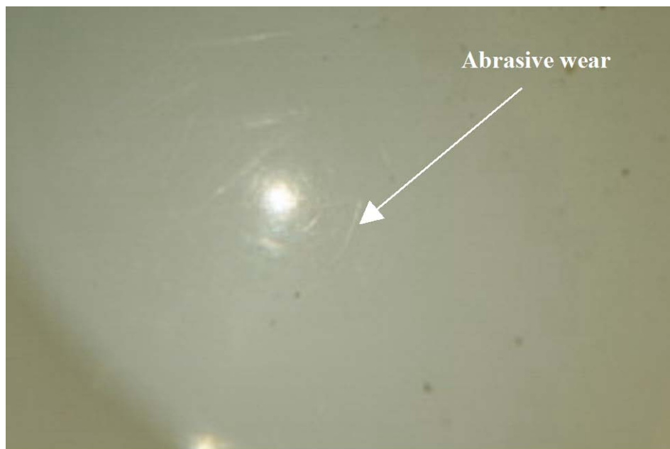
Figure 28: Wear inside the cup
