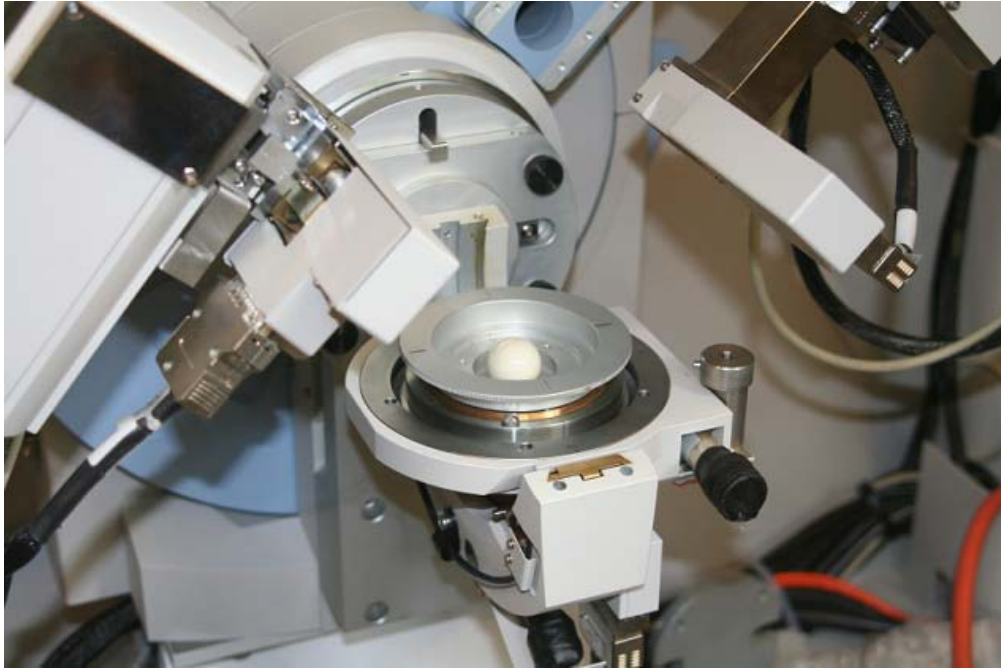
Figure 25: Specimen inside the diffractometer
