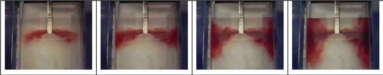
Figure F.1: Old SEN (1060mm width, 150mm submergence depth, 1.1 m/min full-scale cast speed) snapshots
