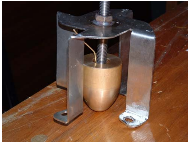
Figure 3.6: Application of dye through the stopper – hole drilled through stopper
