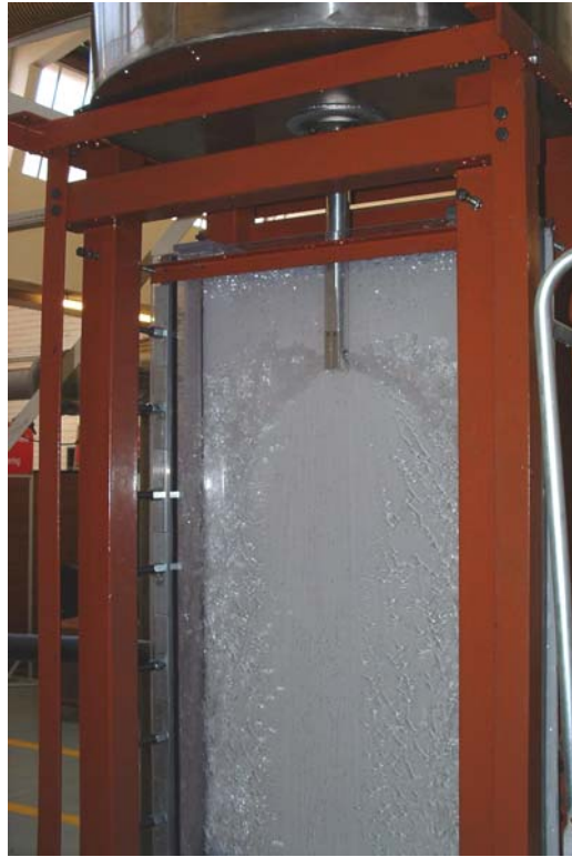
Figure 3.9: Water model being filled up: SEN nozzles exhausting in the air
