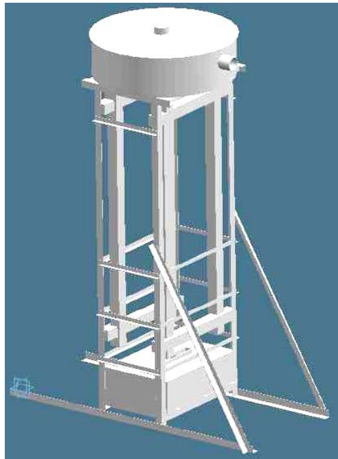
Figure 3.3: General layout of water model (top tank, frame and bottom tank – Perspex mould not shown)
