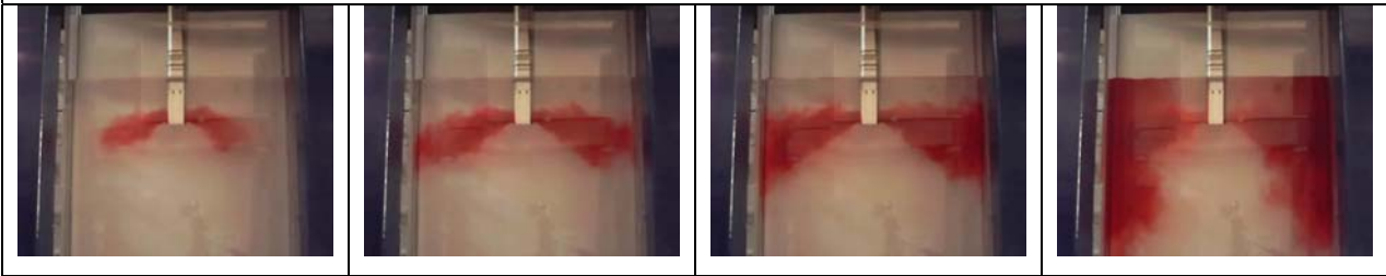
Figure F.4: Old SEN (1060mm width, 80mm submergence depth, 1.0 m/min full-scale cast speed) snapshots
