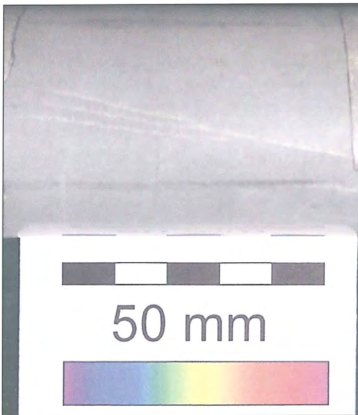
Figure 4.3.13 Tested lava specimen, showing only a few fractures.
