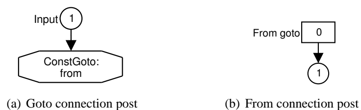
Figure 3.10: Connection post implementation
